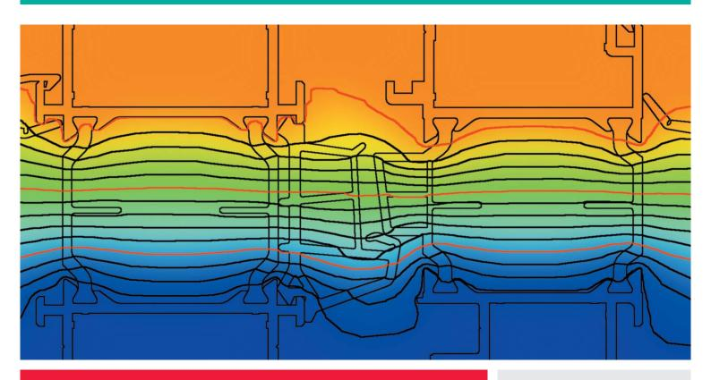
flixo produces thermal-hygro analyses of the component and facade cross-sections. It has been developed by architects, computer scientists and physicists for architects, planners, energy consultants and building physicists.
